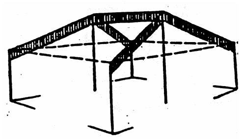
Construction fence at least 2 (two) feet wide (in "international orange" or other contrasting color) shall be assembled to represent the height, bulk and mass of proposed structures. Netting must be supported by stakes or wires strong enough to accurately outline the entire building perimeter and height. A site plan showing the location of story poles shall be submitted to planning staff
