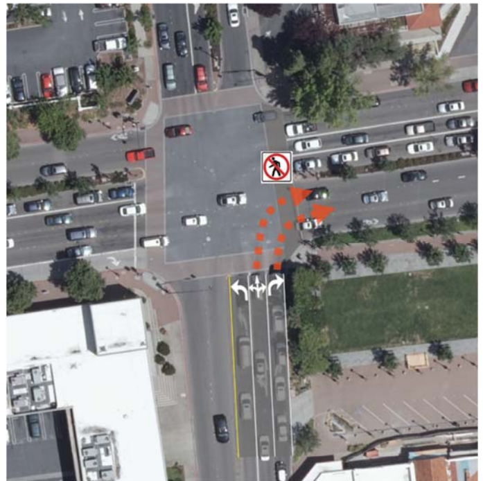
Figure 50: 2nd Northbound Right Turning Lane
