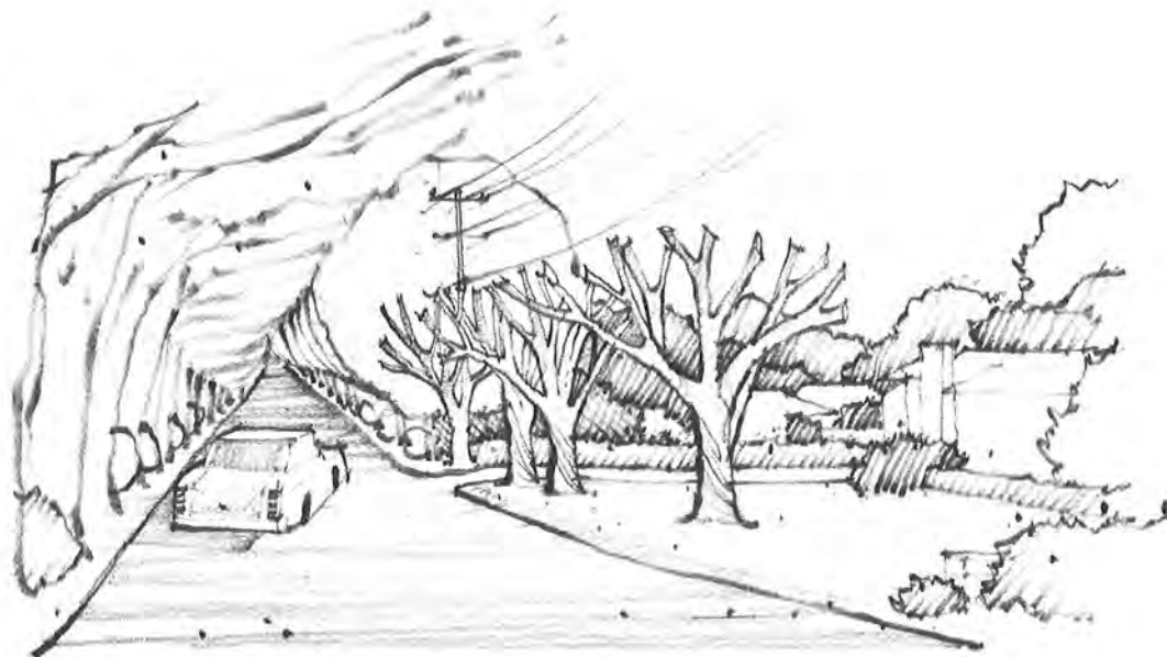
Incorrect power line clearance—trees are ruined and quality of street is degraded.
