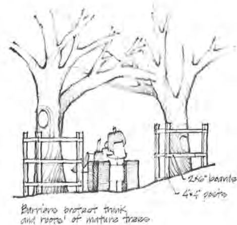
Tree protection barriers for use during site construction work.
