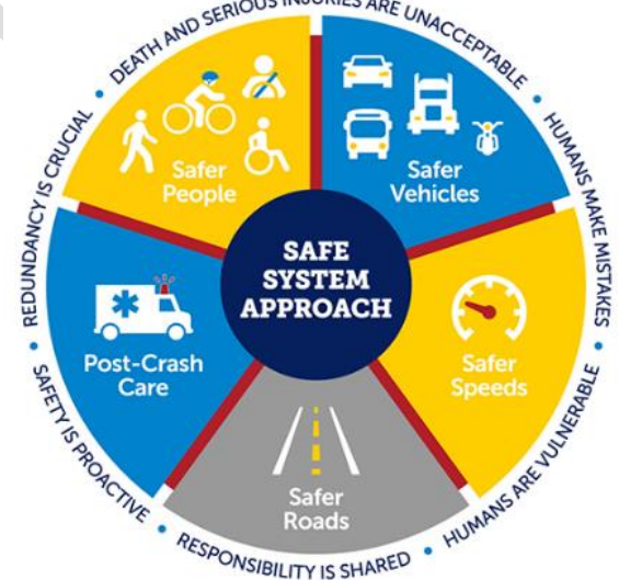
Figure 2. Principles of a Safe System Approach Source: FHWA
