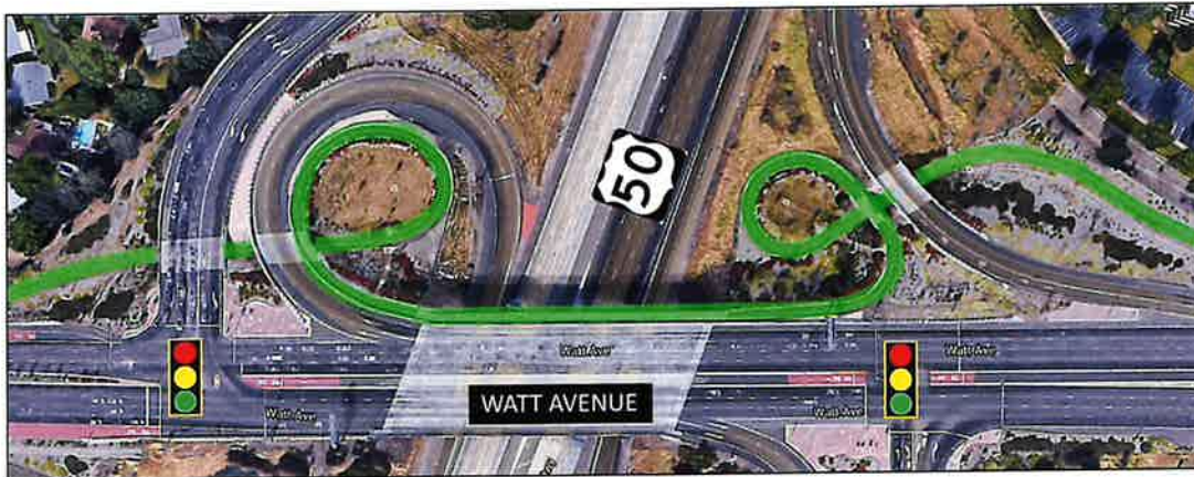
Figure 4-23: US-50 / Watt Avenue interchange – fully grade-separated path
