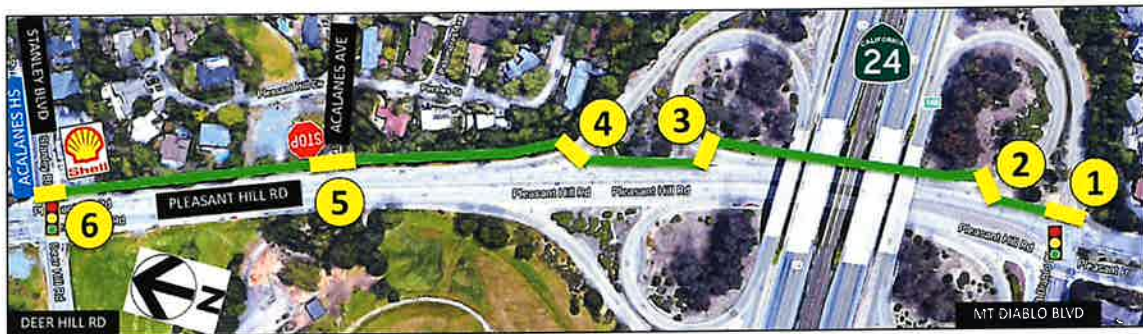
Figure 4-22: Concept for east-side cycle track or shared use path through interchange
