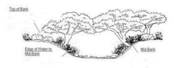
**Zone A:** Edge of active channel, at toe of slope to mid-bank.
