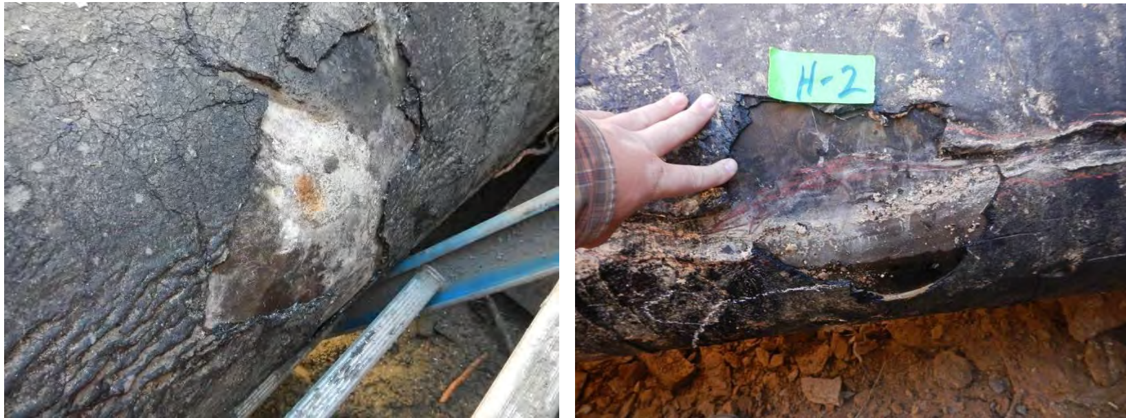
Figure 12. Photographs showing the presence of calcreous deposits in areas where the coating disbonded.
