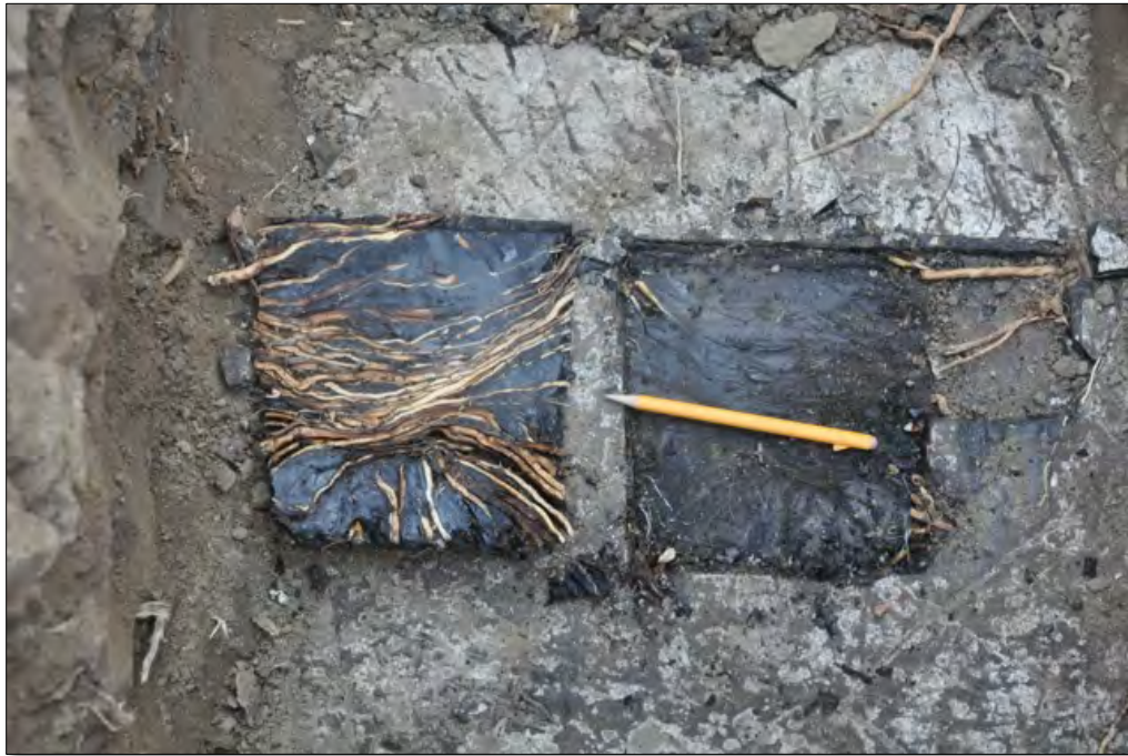
Figure 30. At dig site RWVC-44-13 (RWVIM-100-13) (Palm tree) a 6-inch square sample of coating was removed.
