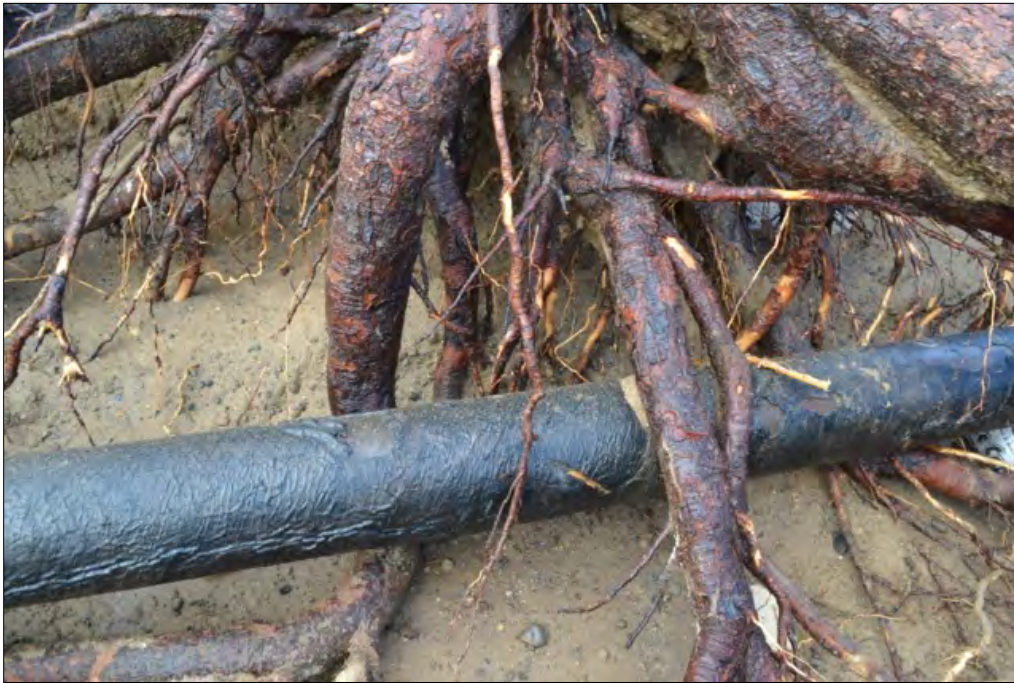
Figure 22. A young Deodar cedar at dig site RWVIM-92-13 interacting with an 8-inch pipe.
