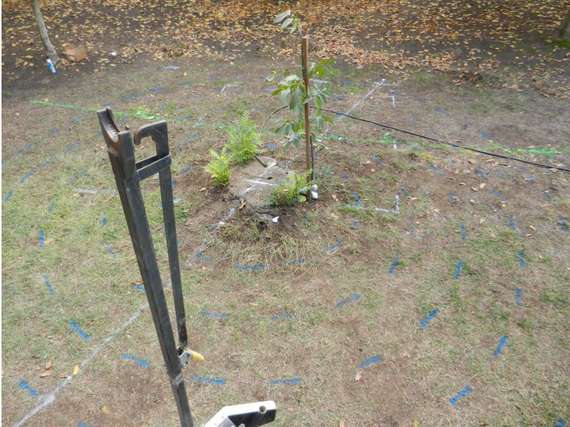
Figure 1. Looking downward and toward the south southwest at walnut stump and plot. Note white line bisecting trunk which was start stop line. Blue lines are scan lines. White box is excavation location and green line is predicted pipe location.
