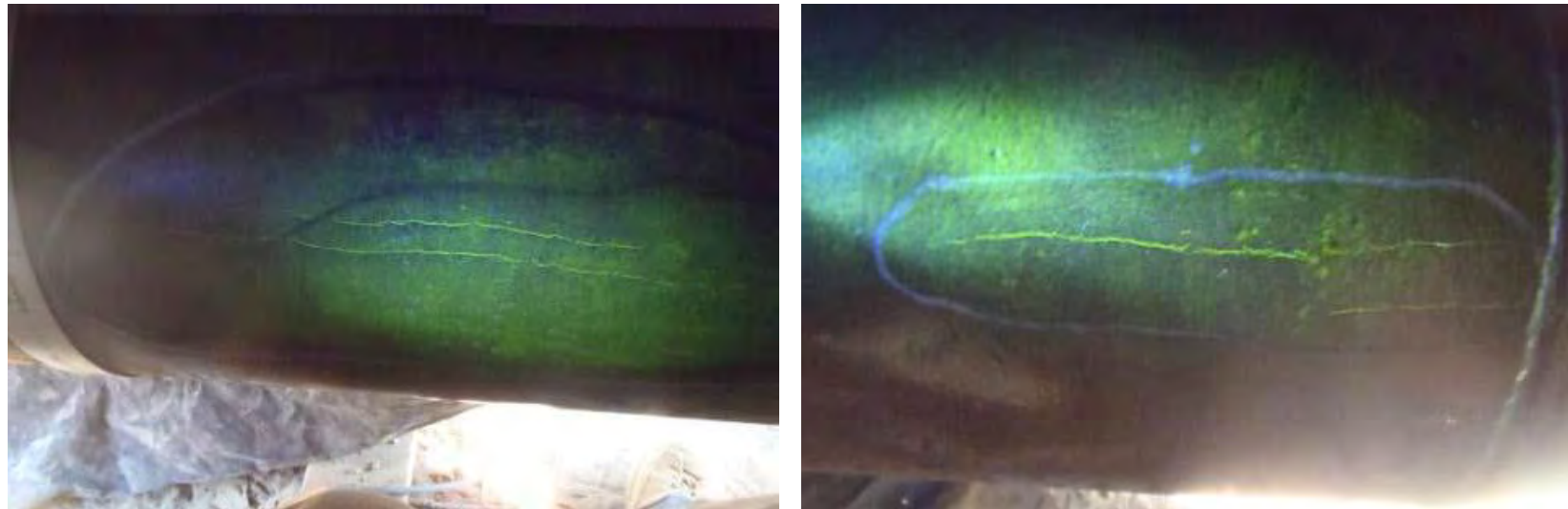
Figure 8. Photographs, provided from Dig RWVIM 89-13, showing representative linear indications identified using wet fluorescent magnetic particle inspection.
