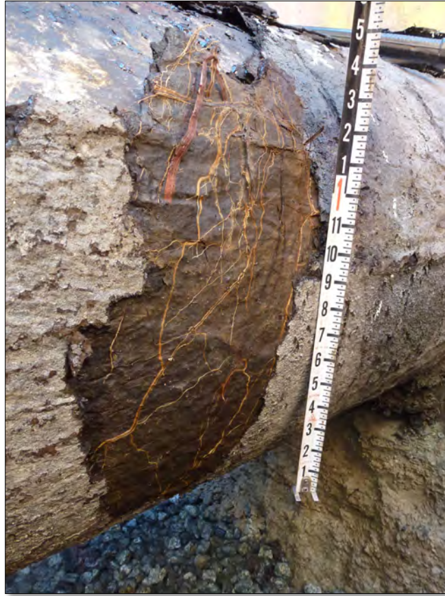
Figure 11. Dig site 132-8 fine roots are growing between the layers of the HAA coating.
