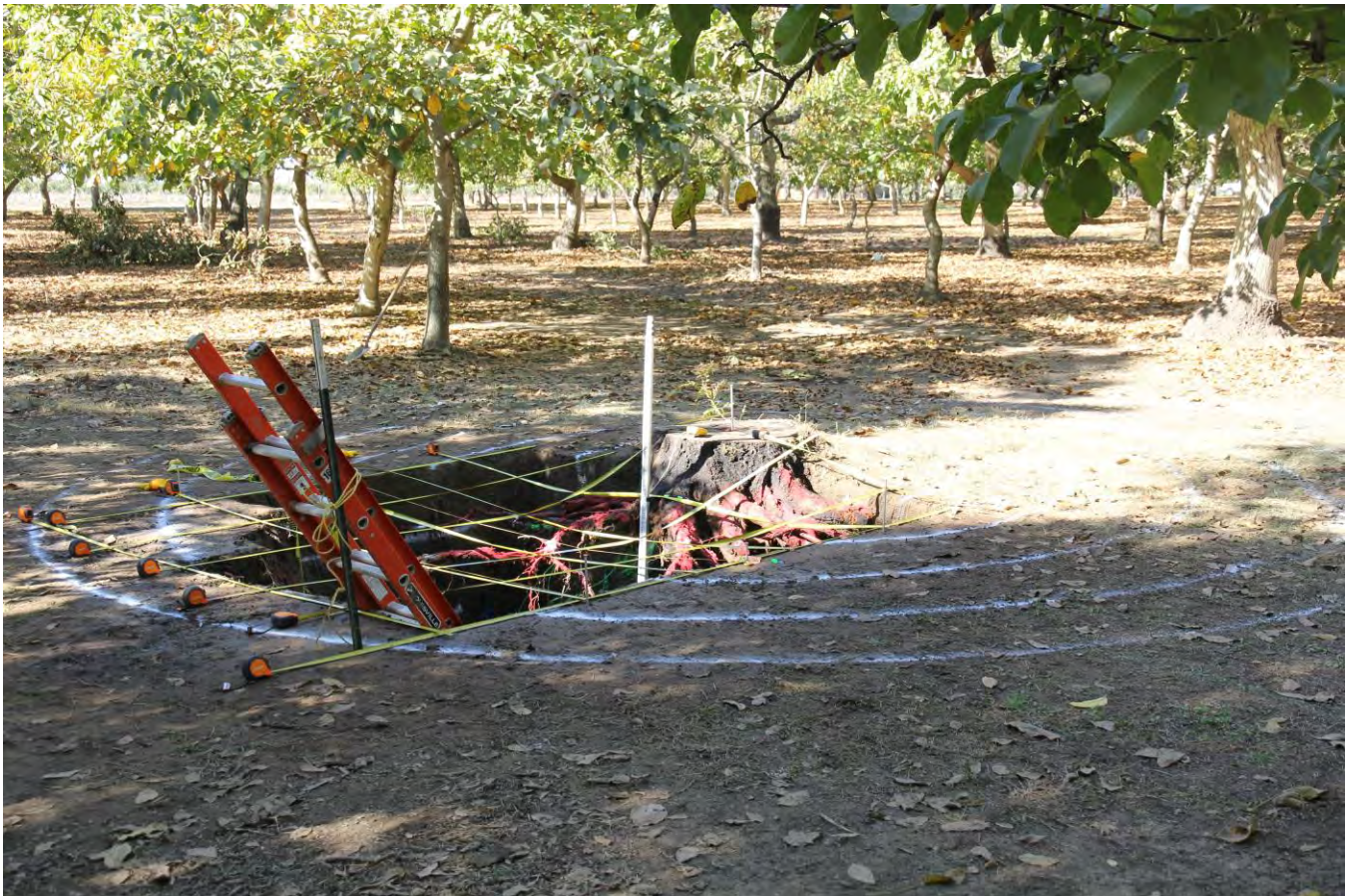
Figure 6. The walnut tree stump at Lockeford. The circular lines were scanned with GPR to map the entire root system. The trees in the orchard were of varying ages and sizes. The excavated tree stump was similar in size to the largest tree in the background of the photo.
