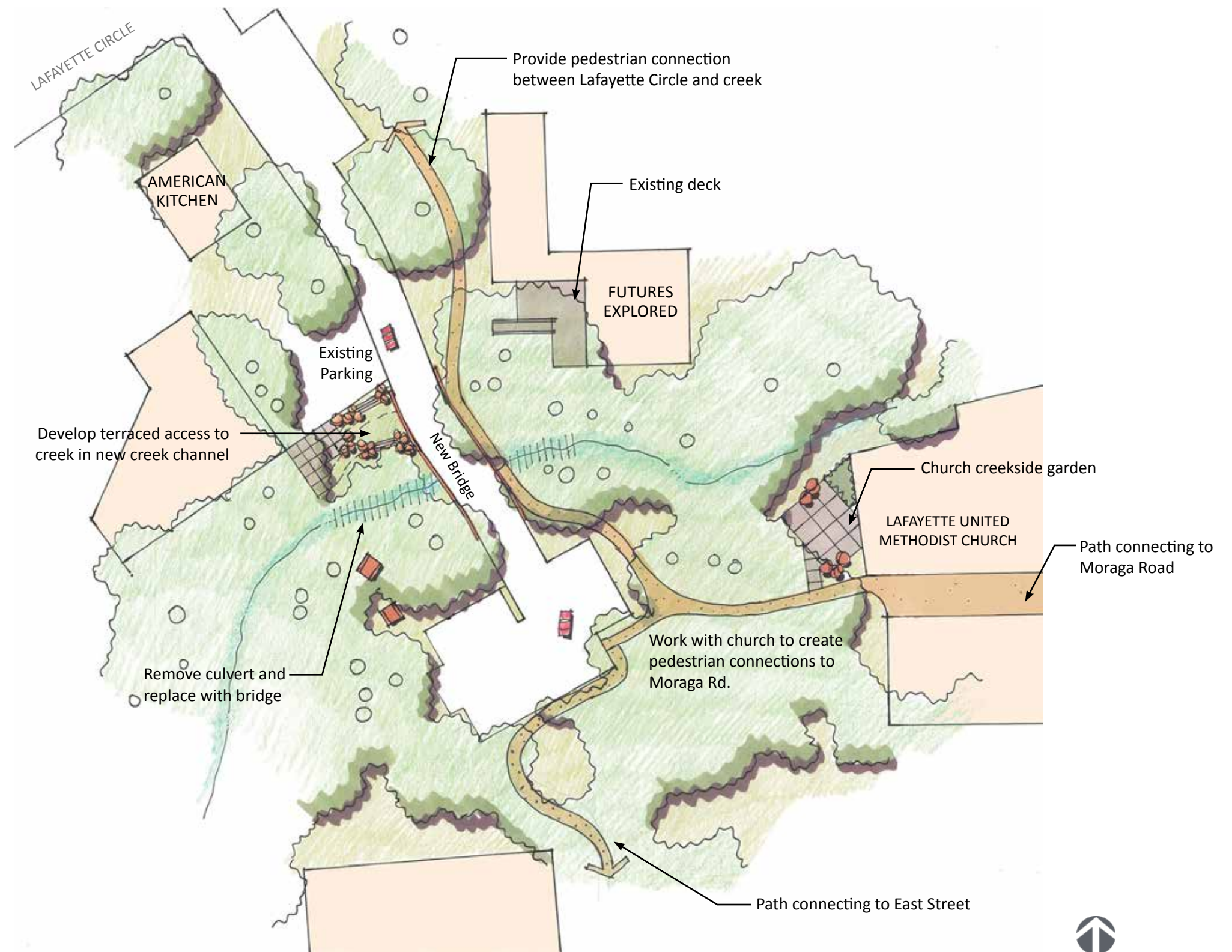
Figure 4-8: Plan View - Restore natural creek by removing culvert under a portion of the parking lot
