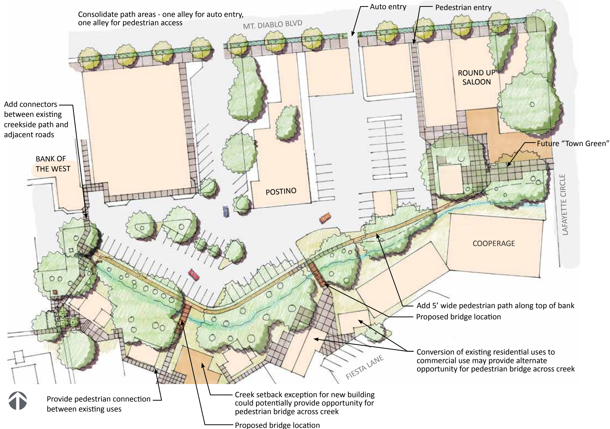
Figure 4-2: Plan View - North Reach improvements
