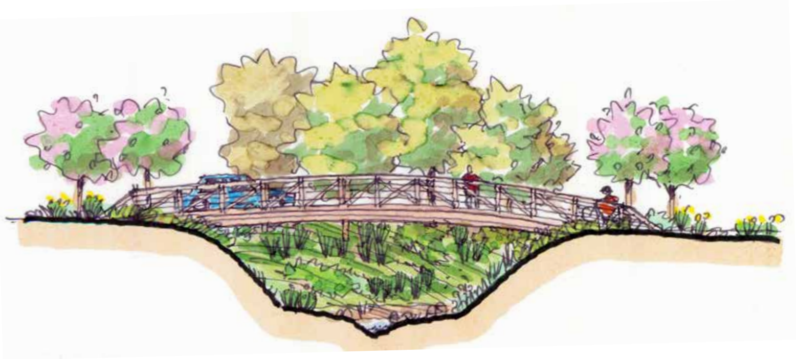
Figure 4-10: Replacing the culvert with a bridge would allow for restoration of the creek channel. (N.T.S.)
