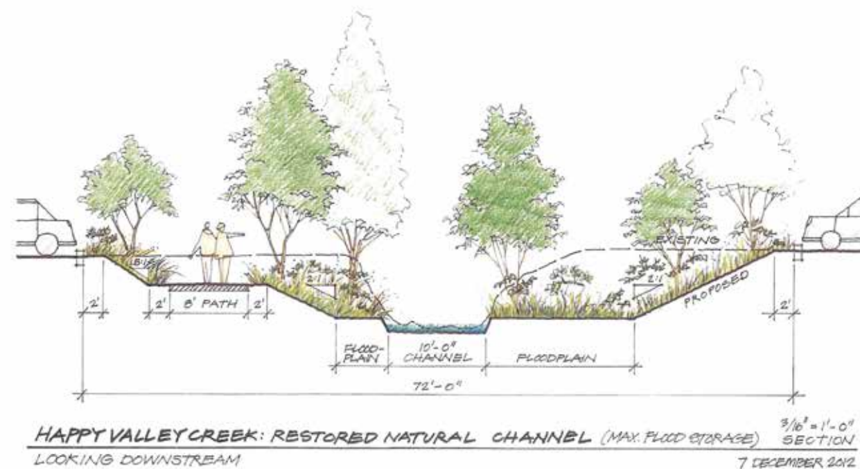
Figure 8: Restored riparian channel concept sketch Source: Restoration Design Group
