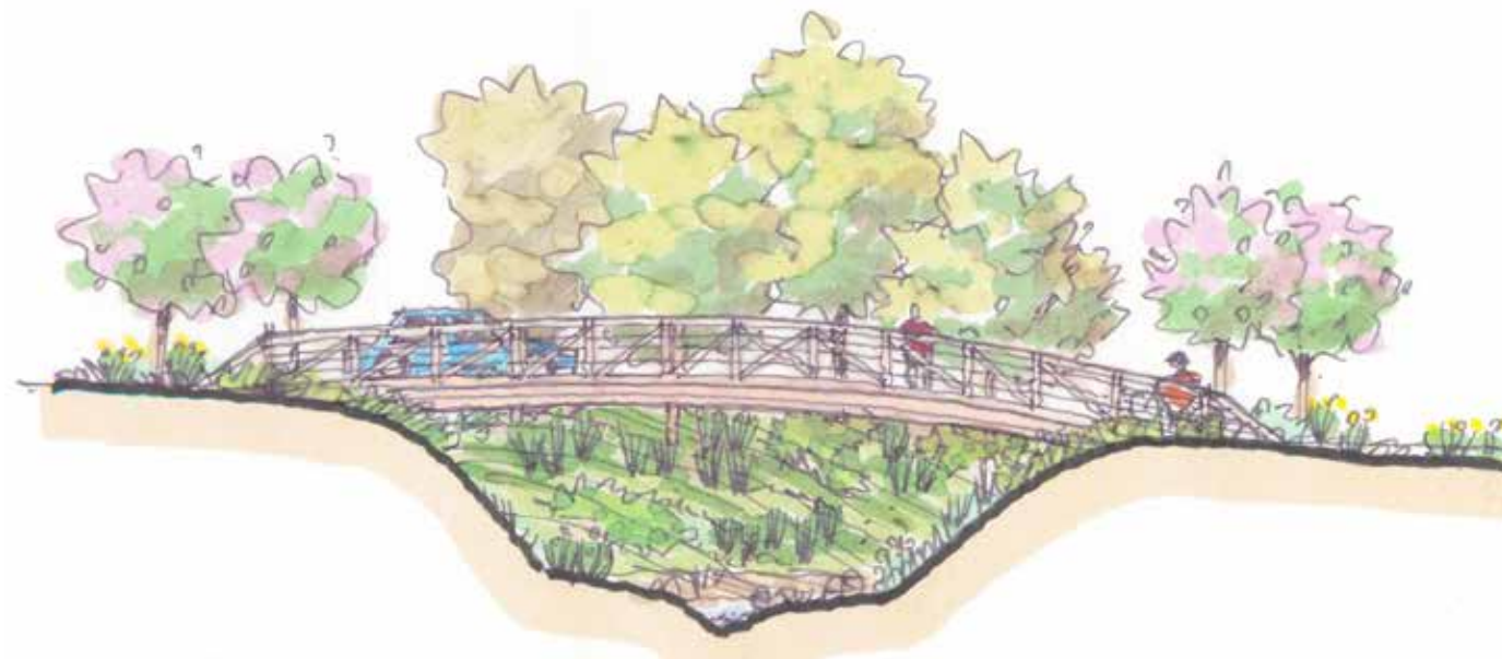
Replacing the culvert with a bridge would allow for restoration of the creek channel, improving habitat value and aesthetic value, but parking spaces would be lost
