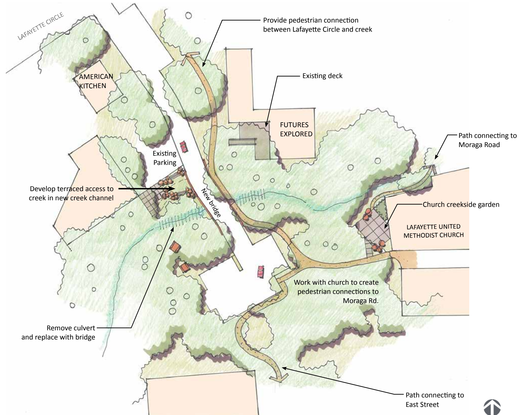
Plan View - Potential to restore natural creek by removing culvert under parking access
