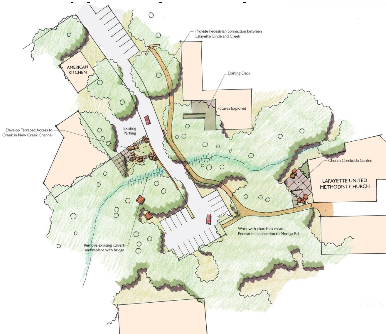
SOUTH REACH - LAFAYETTE CREEK AT METHODIST CHURCH PARKING LOT REPLACE CREEK CULVERT WITH BRIDGE AND ADD PUBLIC ACCESS TO CREEK
