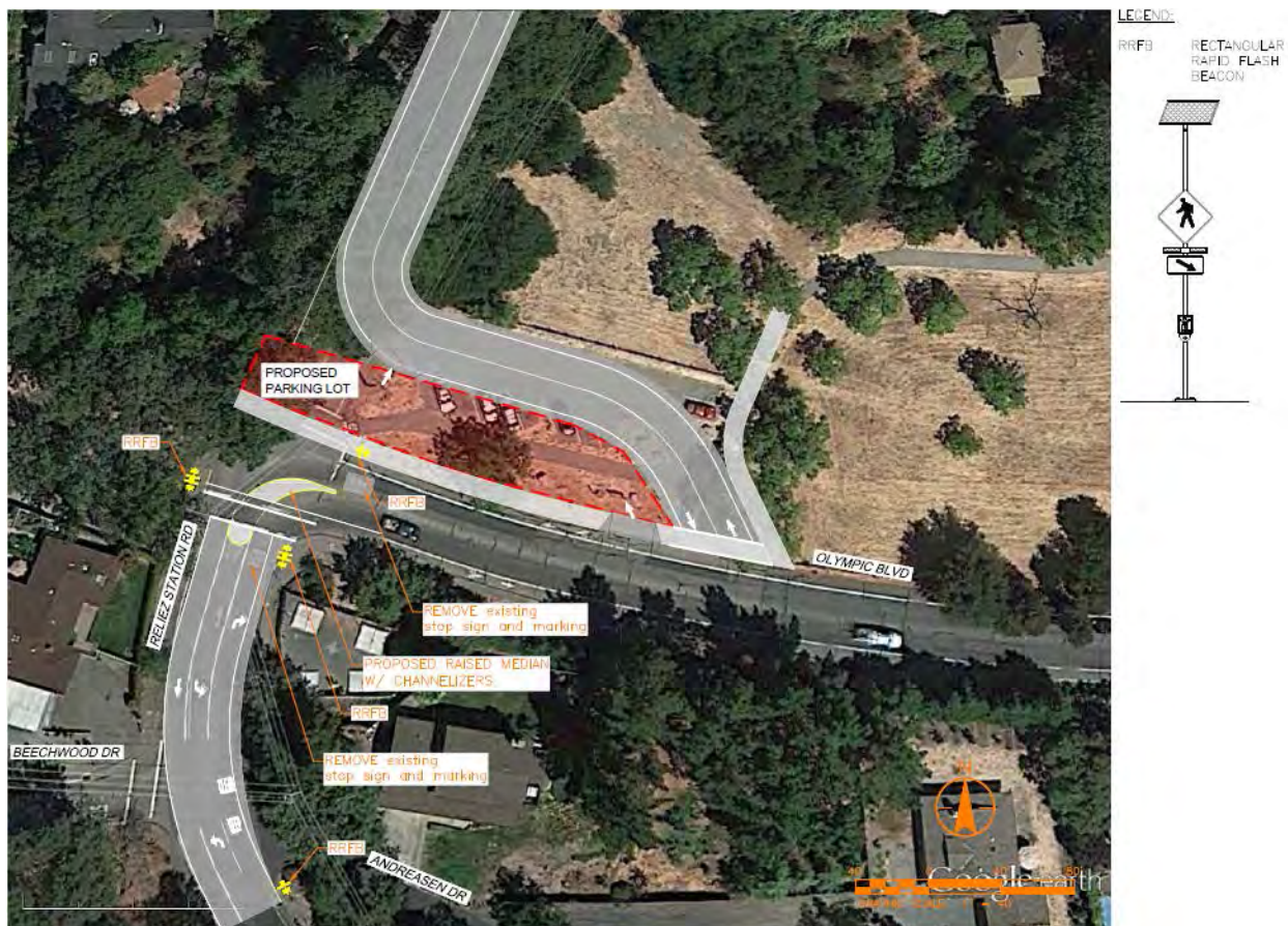
Figure 6: Reliez Station Road & Olympic Boulevard Alternative #1-C: Free NB Right and WB Left with a Raised Median and Relocated Parking Lot
