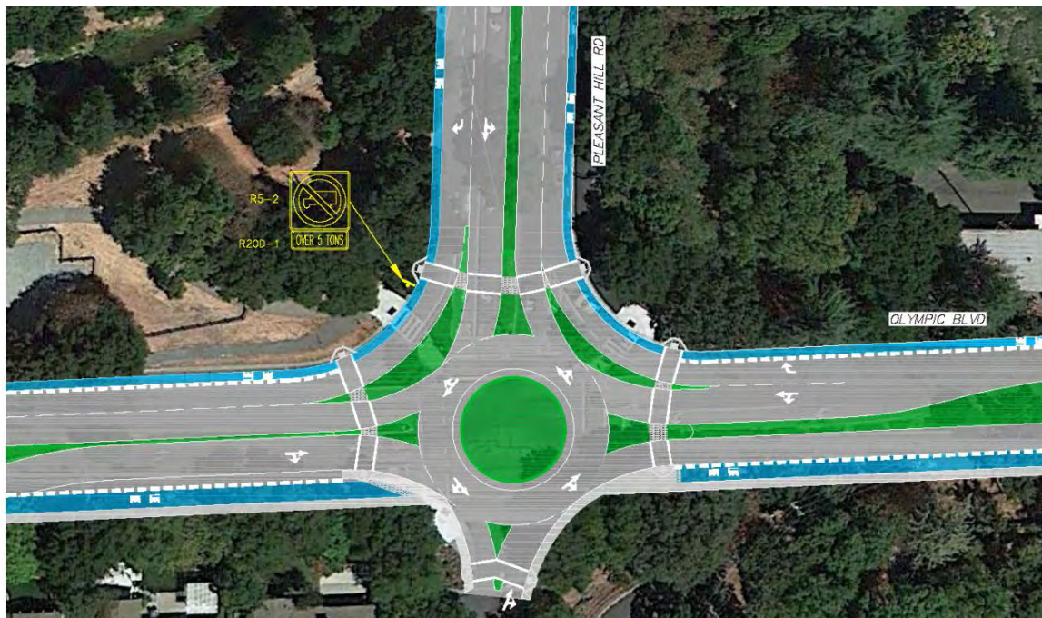
Figure 3: Olympic Boulevard & Pleasant Hill Road Alternative #2: Roundabout
