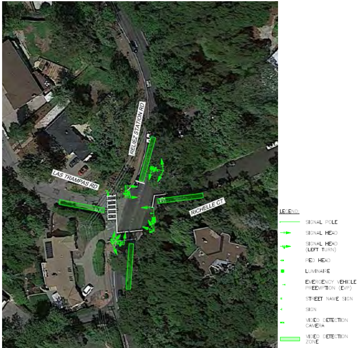
Figure 11: Reliez Station Road & Las Trampas Road / Richelle Court Alternative #2: Traffic Signal
