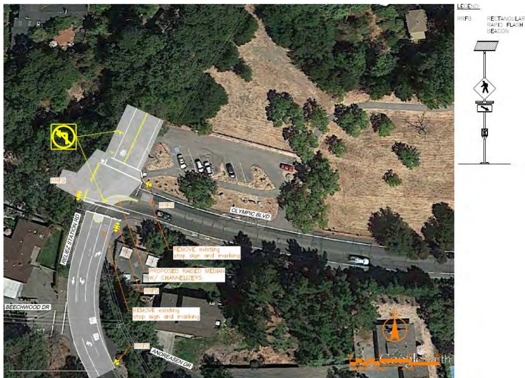
Figure 5: Reliez Station Road & Olympic Boulevard Alternative #1-B: Free NB Right and WB Left with a Raised Median
