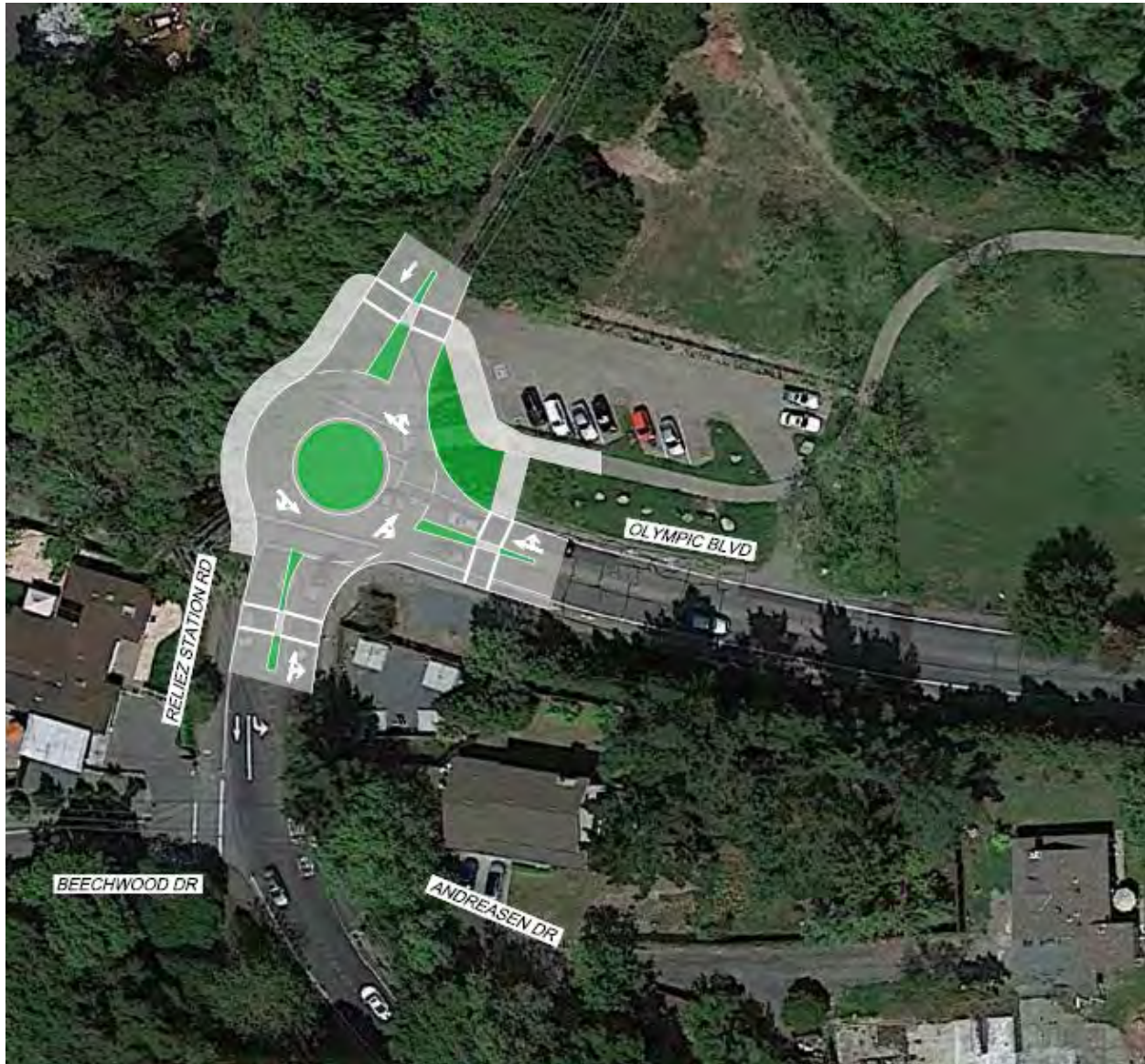
Figure 9: Reliez Station Road & Olympic Boulevard Alternative #3: Roundabout
