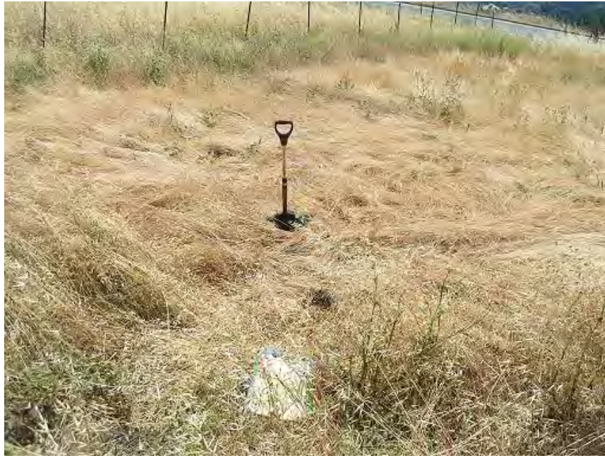
Photograph 1. Seasonal wetland in south-central portion of Property facing south towards Deer Hill Road showing the location of T-1. Shovel marks the location of sample point T-1b and field notebook the upland boundary (T-1a). Note the nearly pure stand of matted perennial ryegrass (FAC) in the mapped feature.
