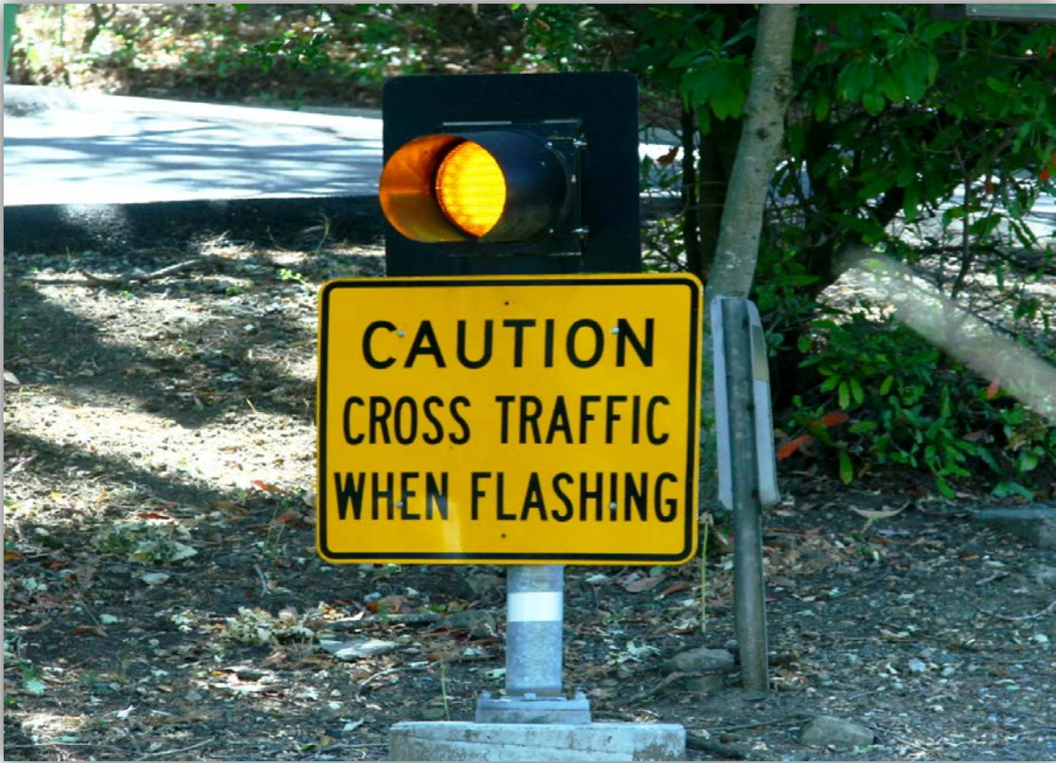
Figure 1: Flashing Beacon Warning of Cross Traffic Ahead
