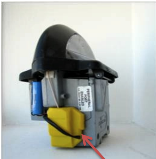
Meter with Streetline Meter Monitor Installed.
